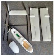
Insert the stabilizer rod into the hole in the center end of each wing and slide wings together. The wing spar can be verified on an assembled aircraft by observing the green color when looking through the cutout in the top of the wing assembly. If the wing spar is not present, you will observe a red color in the wing cutout.
