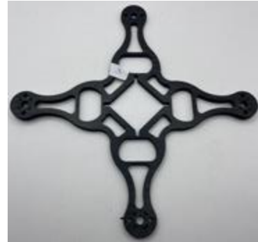
Thickness: 5.15 mm Material: Carbon Fiber Label: 3
