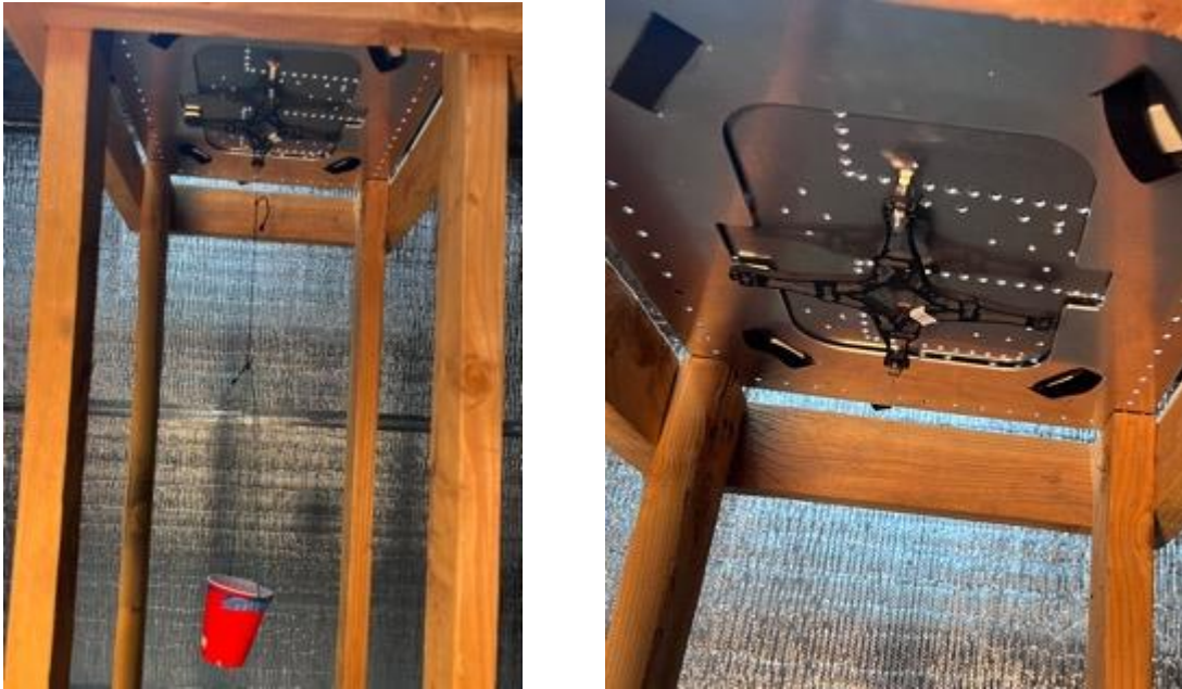
Figure 4: The wooden test frame with the drone frame and metal plate placed on top. The hanging weight is shown that was used to add weight to the data frame.
