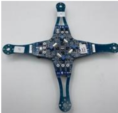
Thickness: 2.41 mm Material: Fiberglass Label: 4 & 5
